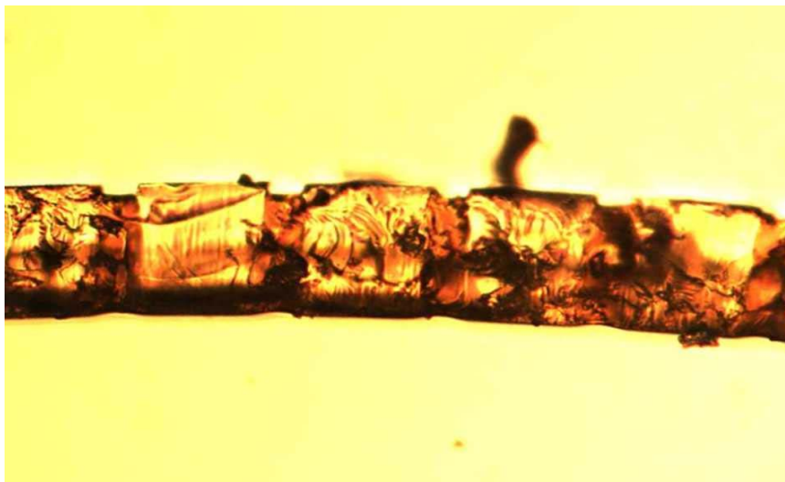
Figure 5.13. Polarized light micrograph showing cross-section of HEA film containing optimized 2-component Eosin Y photoinitiator system. Illuminated for 1 mintue with 150 W xenon lamp through PET film containing 50x100 \mu\text{m} gold electrode spacing.
